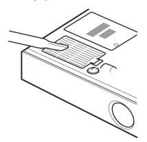
When it becomes difficult to remove the dust from the filter with a vacuum cleaner, remove the air filter and wash it.
