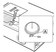
**3** When opening/closing the lens protector, turn the groove of the adjuster with a coin.
