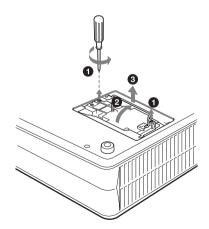
5 Insert the new lamp all the way in until it is securely in place (1). Tighten the two screws (2). Fold the handle (3).
